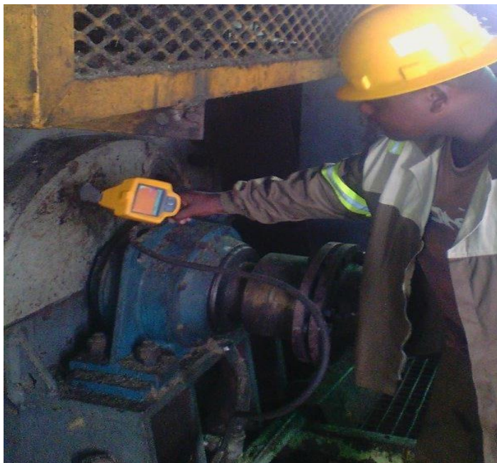
Figure 4: Temperature monitoring using a handheld meter
