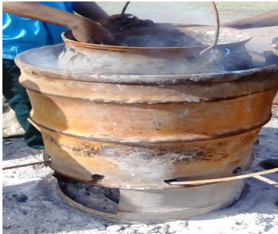
Figure 1: A 200 L steel drum used as the furnace. Melting charge is loaded in the cast iron pot. The rectangular opening at the bottom serves as tuyere. The furnace does not have a lid.
