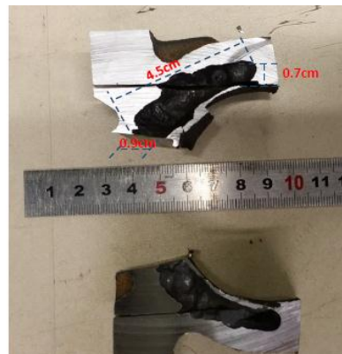
Figure 2: Gas defect at Foundry 2
