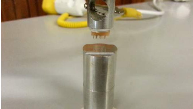
(i) Gripper aligned and ready for placement operation
