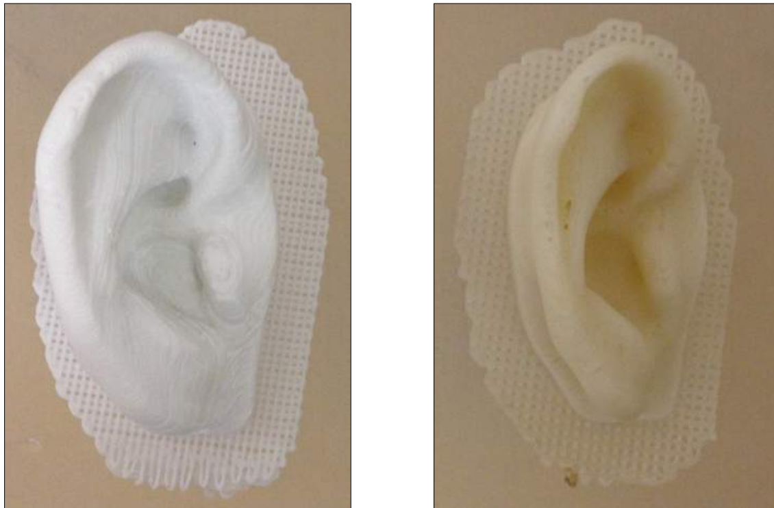
Figure 9: Finished prototypes of the ears with PLA (left) and ABS (right) materials
