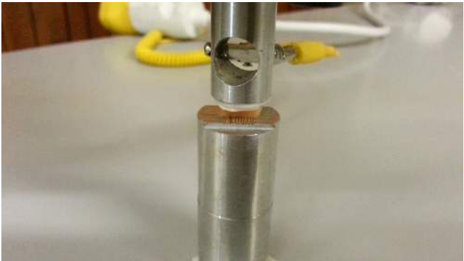
(iii) Gripper raised until preload force of 0N is read by force sensor
