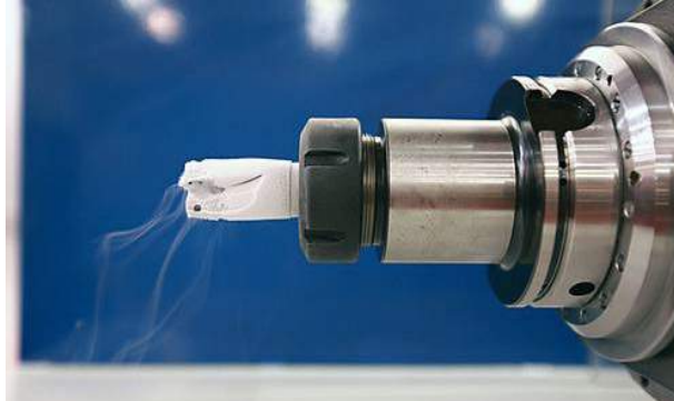
Figure 10: Cryogenic minimum quantity lubrication & through spindle cooling system [29].
