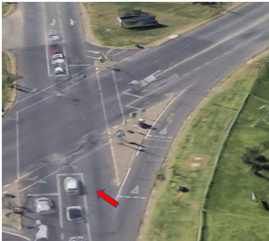
Figure 3: Showing the excluded right turning lane group [13].
