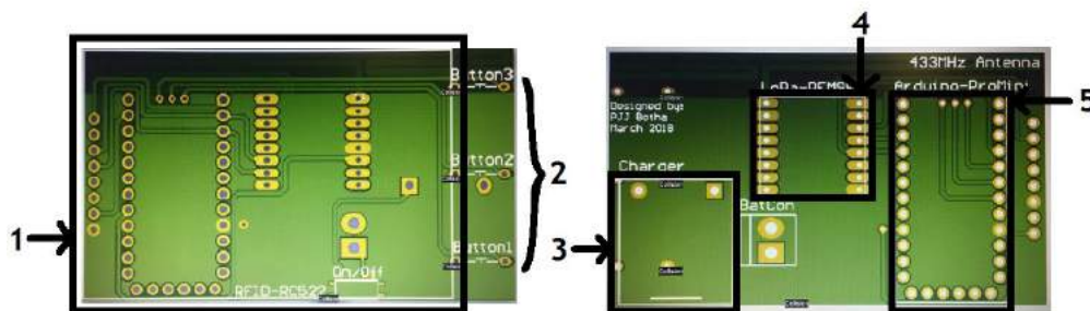
Figure 4: Front and back view of the developed PCB for sensor
