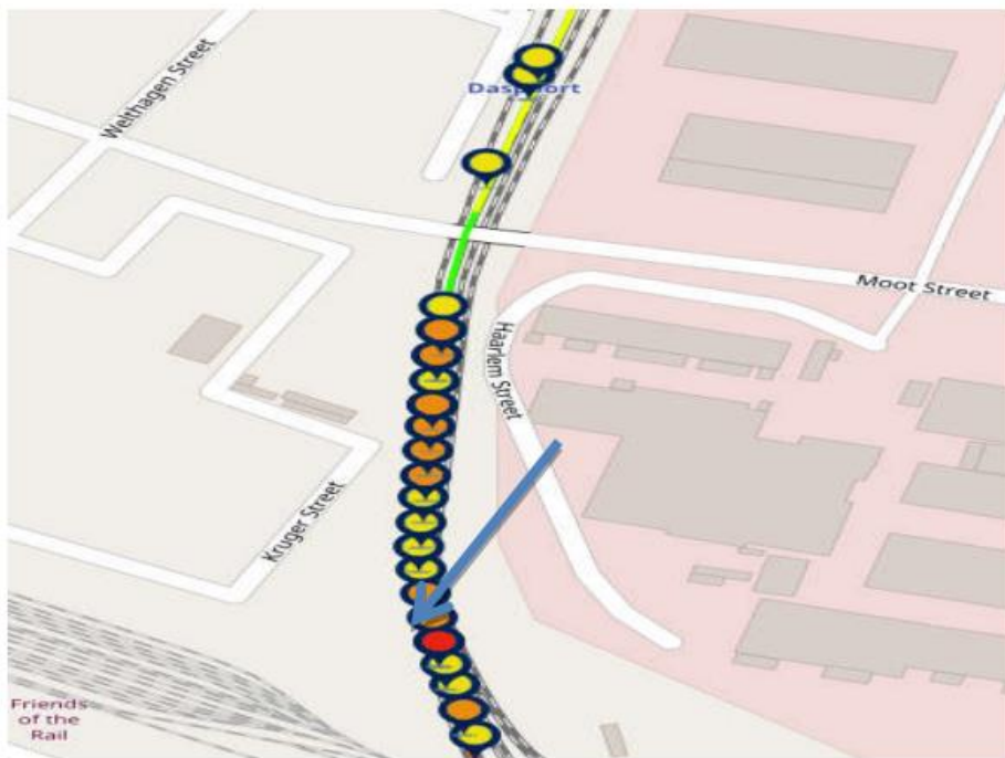
Figure 10: RED class defect noted from Pretoria to Koedoespoort
