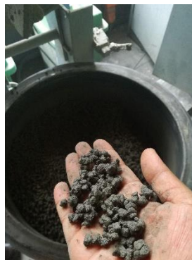
Figure 4: Poor paste for water to cement ratio of 0.24.
