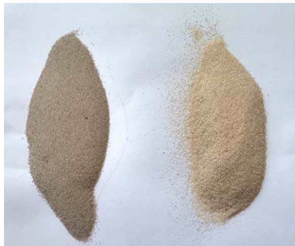
Figure 2: Silica sand samples - waste sand from sand printing of furan-bonded sand cores (left), virgin silica sand (right)
