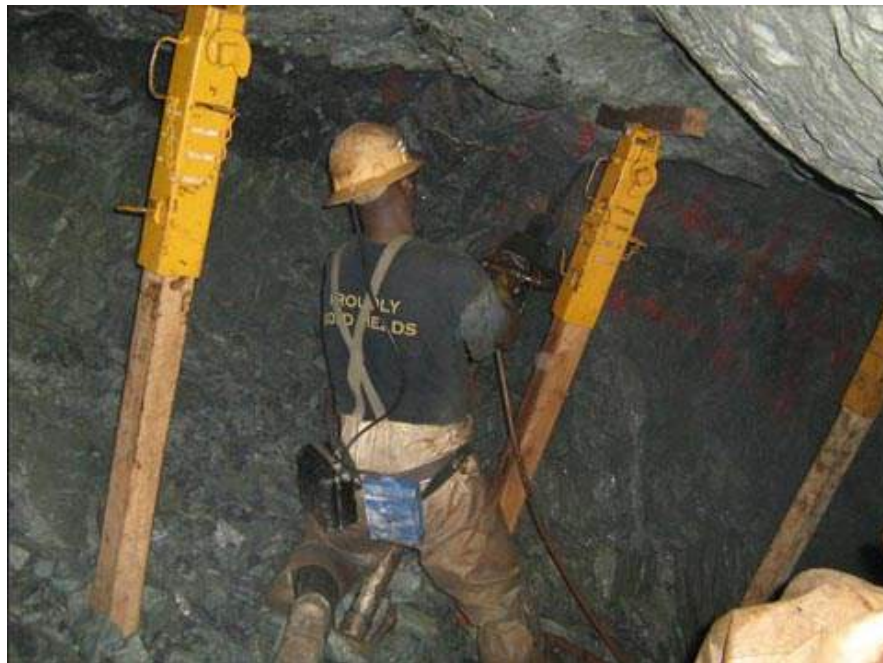
Figure 2: Roof Support Systems
