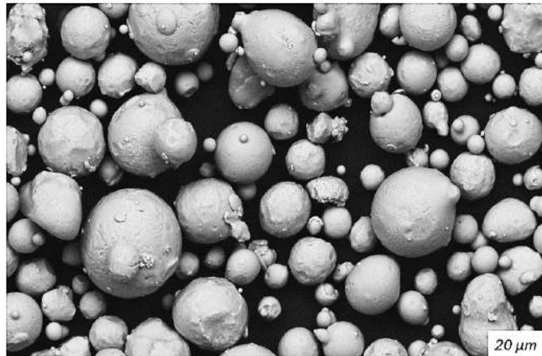
Figure 2: SEM Image Showing the Morphology of 304SS Powder Particles.
